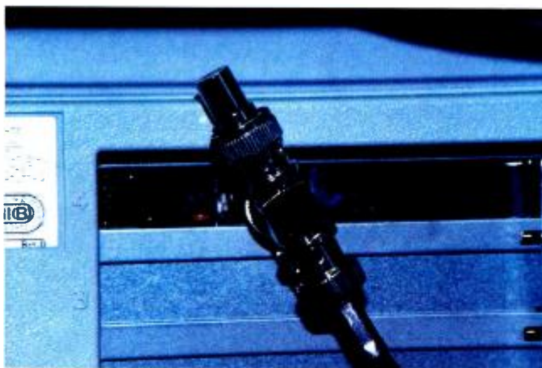
Note the 50 \Omega terminator connection to one side of the BNC "T."
